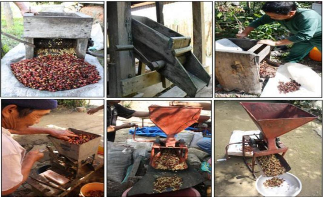
Figure 12 . Improved wooden coffee depulpers (above) and locally fabricated metal depulpers
